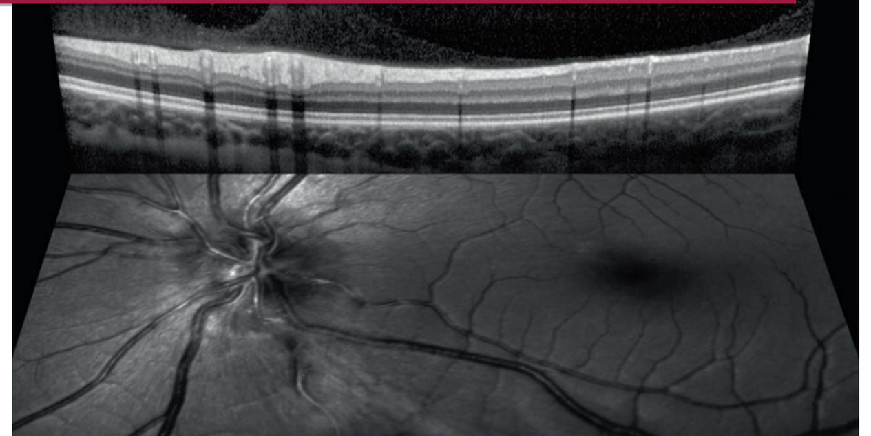
The patented TruTrack Active Eye Tracking uses a second laser beam to actively track the fundus during OCT scanning to minimize motion artifact. The precise alignment of blood vessels from fundus image to the corresponding OCT scan facilitates unsurpassed dynamic visualization.
