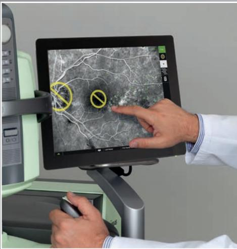
Touchscreen for device operation, placement of plan spots and direction of aiming beam.
