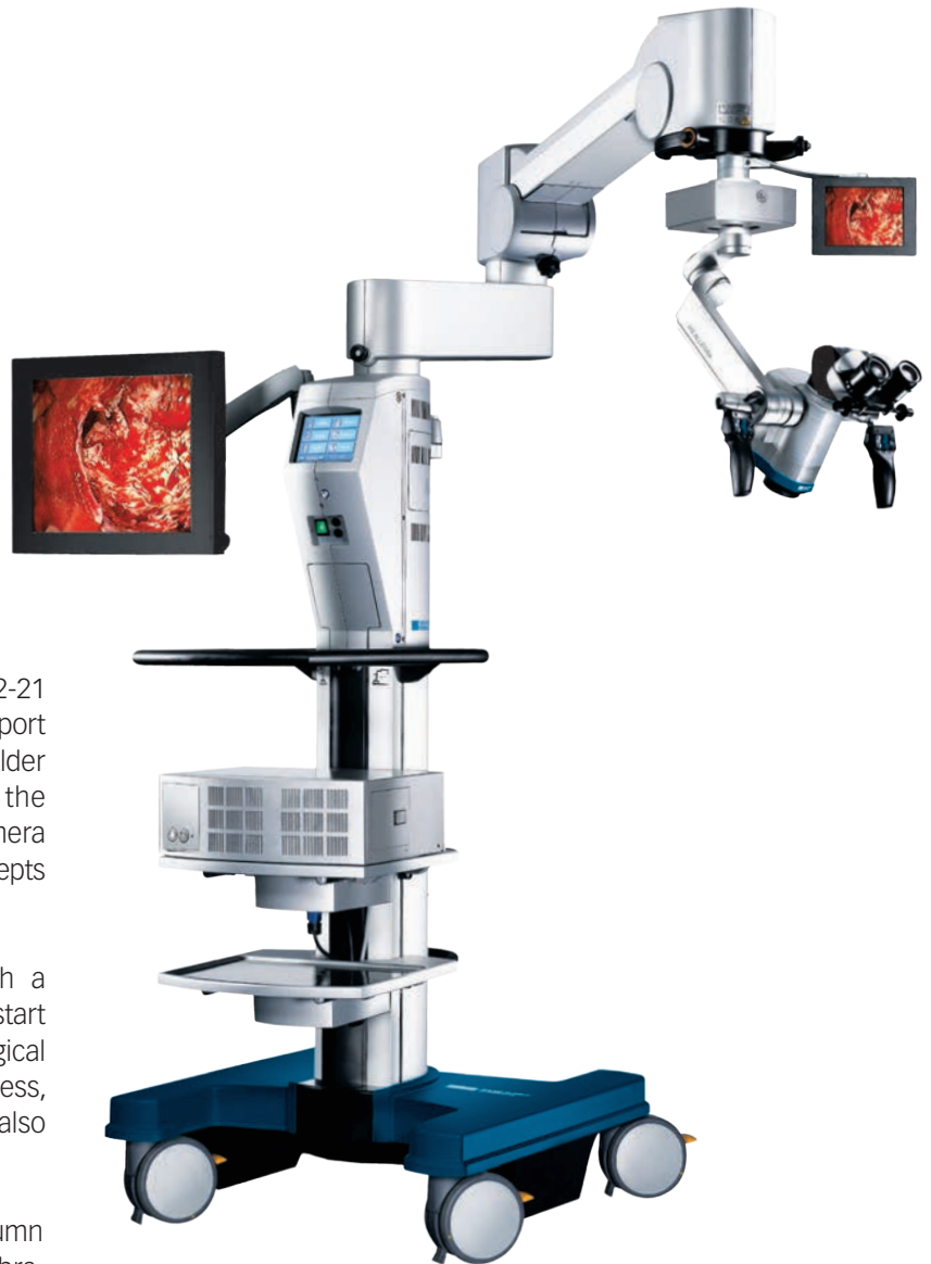
HS ALLEGRA 500 on floor stand FS 2-23 with 300 W xenon illumination
